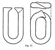
In making chains, do not weld two single ' links and then one between them. Weld a link on the end of the chain and keep repeating until finished.
