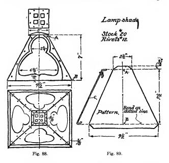
87 is shown the drawing which does not need explanation. The drawing for the pattern is shown at Figure 88 and the pattern for one section at Figure 89. In developing the pattern which is very simple the top drawing, Figure 88, represents the shade which should be drawn full size. The length from A to B is then laid off on the center line of the pattern, which in this case measures  $7\frac{1}{2}$  in. The top and bottom of shade shows a return of  $\frac{3}{8}$  in. which
