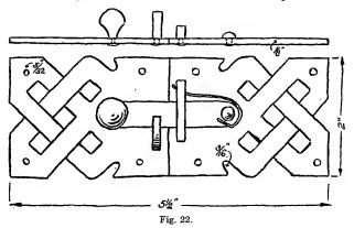
the square holes come in the design. The plates are then heated and a square punch is used to drift out the holes. The outside edges are then cut. The plate is heated and with a square punch the metal is set down to give it the interlaced effect as shown in Figure 23.
