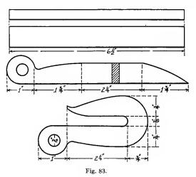
$6\frac{1}{2}$  by  $\frac{3}{4}$  by  $\frac{3}{8}$  inches. To form the eye one end is heated and shouldered back one inch from the end, by hammering it on the anvil as shown in Figure 84. The eye
