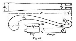
lug shown on the drawing is to be made and riveted into the top of the plate. The hammer is then placed over the lug, and the lug is drilled to conform to the drilled holes in the hammer.
