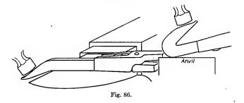
point is next drawn out and then the hook is heated in the center. It is cooled each side of the center and hammered over the horn to bend, then on the anvil as shown at Figure 86. A piece of  $\frac{3}{8}$ -in. flat iron is set on the inside of the hook and the hook hammered to fit the iron. This leaves the opening of the hook uniform and just the size required. See Figure 87.
