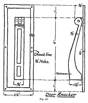
chisel is used for cold work and a longer one for hot work. The chasing can be done while the metal is cold. If it is to be very deep or wide the plate is heated and a longer chisel is used. The lug at Figure 42 is made and riveted into the plate. The top of the hammer is filed to straddle it. A hole is then drilled and a rivet put thru. Holes are drilled around the edge of the plate for screws or nails.
