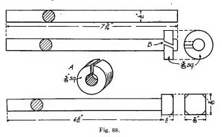
Figure 88 shows a welded bolt head. After the stock is cut to proper length, the collar for the head is made. It is heated and hammered over the horn of the anvil to make it round. The end of the collar is now cut off on the hardie, cutting clear thru from one side and giving it a bevel. The other end is cut from the opposite side giving it a bevel also. See drawing at A. The collar is driven on the end of the bar while
