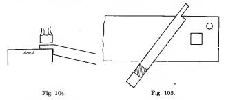
of the anvil and hammering to form the shoulder for the eye. See Figure 105. It is then turned again to the left hand and hammered down for the last shoulder.
