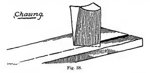
around the edge of plate. In doing this a short, light chisel is used. After lines are traced on the plate with a slate pencil the chisel is set on the line and struck with a light hammer; at the same time it is drawn towards. the worker with the lead corner of the cutting edge directly on and above the line.
