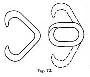
See Figure 72. Notice in the drawing that the hooks at the open end of the link are not very long. They should not be made longer than shown.
