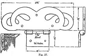
The hinge can be made any length desired but should be carefully proportioned; the eye can be made loose or welded. In welding a hinge-eye the lap should always be on the back. Note the drawing of the eye
