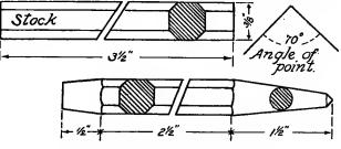
Fig. 120 (above). Center Punch. Fig. 121 (below).
