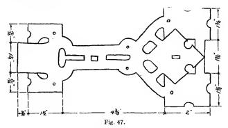
At Figure 46 is shown a door knocker hinged at the top. The plate is one piece. At Figure 47 are shown the dimensions of the plate. After the shape of the plate is sketched on the metal, the lines are traced with a chisel. The open work is then cut out, and the outside of the plate is cut and filed. The center leaf at the top of the plate is indicated by forcing the metal down along the top edge of the leaf with a punch, also
