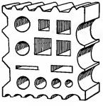
Fig. 19. Cast Iron Swage Block.
