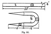
end with a pair of light tongs. The piece is then heated and drawn out to a point; it is reversed in the tongs and the other end is drawn out. The center of the piece is then reheated and bent into shape over the horn of the anvil.
