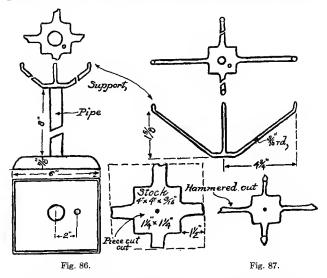
borax and spelter should be applied to the under side, after the base is well heated, as the brass will discolor the iron on the top side. When the pipe is brazed it should be made to stand vertical.
