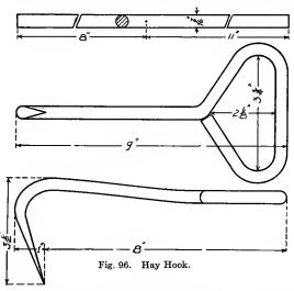
first turned, using 11 inches of the bar. The end is then heated and drawn to a point after which it is bent as shown in the drawing.
