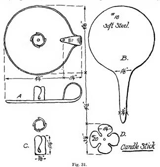
Figure 31, at A, gives the dimensions; at B, is shown the pattern of the bottom in the flat. The bottom is cut from a sheet of soft steel, using a narrow cold chisel. The edge is then filed and bent up about one-quarter of
