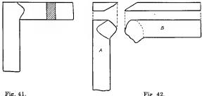
scarfs prepared for a corner weld, using 1" by  $\frac{1}{2}$ " stock. The piece at "A" is scarfed with the ball of the hammer. The one at B, with the face of the hammer. Separate heats are taken and the pieces lapped and welded.
