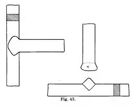
hammered. Notice how wide the scarf is made on the end piece at "A". This is done to cover the other scarf. All flat "T" scarfs are made in this manner.
