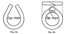
In welding the ring, it is handled in the same manner as in welding links. To find the amount of stock for rings, the inside diameter plus the thickness of stock is multiplied by 3.1416 or 3 1–7. To this is added enough stock for the lap of the weld. For example a ring is required of one-inch stock. The inside measure is 10 inches. Solution:  $(10 + 1) \ge 3 - 7 = 11 \ge 3 - 7 = 34 - 7 + \frac{1}{2}$  inch for welding.
