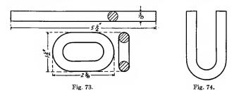
"U" shape. See Figure 74. The ends are now heated and scarfed by setting them on the anvil as shown in Figure 75. The iron is then struck on top with the hand hammer. After each blow, it is moved away from the anvil just a little, giving the end a bevel, so that, when finished, the scarf consists of a series of slanting notches.
