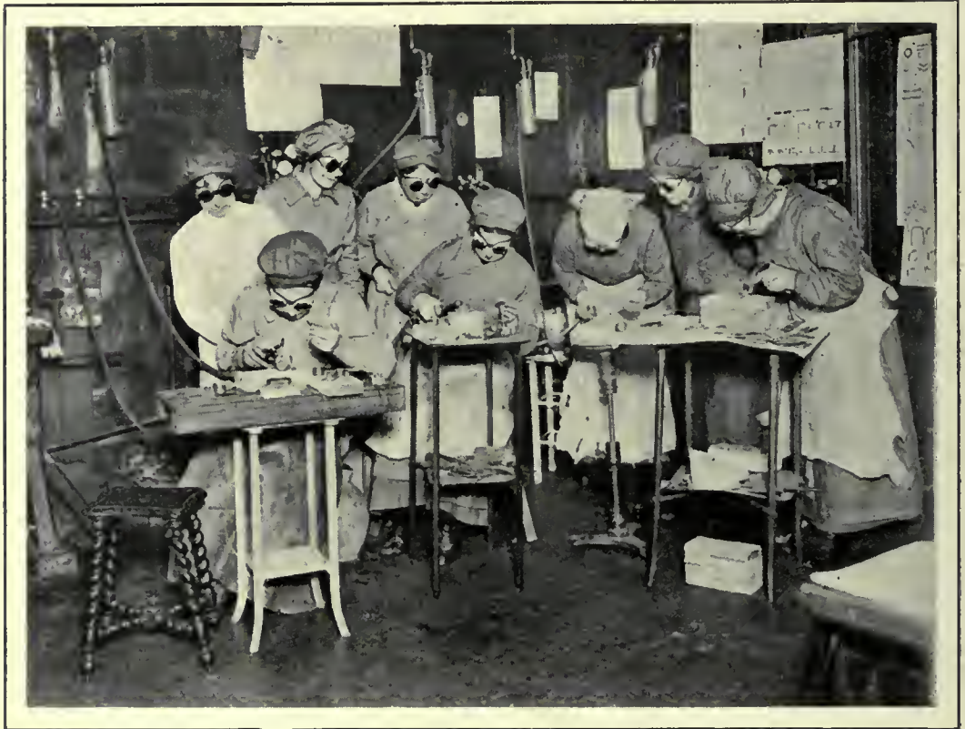
WELDING AEROPLANE PARTS BY MEANS OF ACETYLENE BLOW-PIPES.
