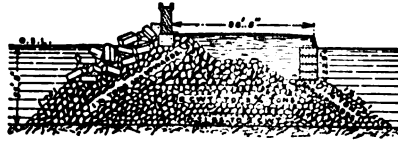
FIG. 5.—Marseilles Breakwater, central portion.
