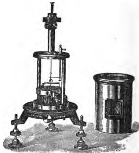
FIG. 7.—Quadrant Electrometer. Dolezalek Pattern.
