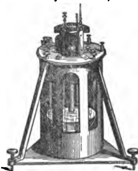
FIG. 6.—Kelvin's Quadrant Electrometer.
