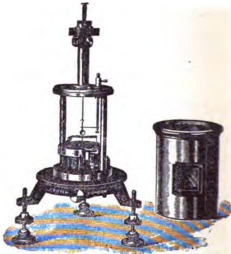
FIG. 7.—Quadrant Electrometer. Dolezalek Pattern.
