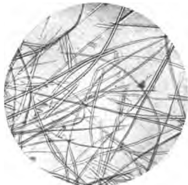
FIG. 11.—ESPARTO. Cellulose. Ultimate fibres of paper making pulp. Typical fusiform bast fibres, with scattered serrated cells of cortex and hairs.
