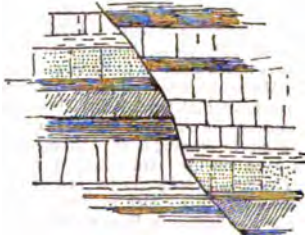
FIG. 1.—Section of clean-cut fault.
