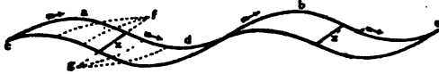
FIG. 13.—Wave track made by the wing in progressive flight. a, b , Crests of the wave; c, d, e , up strokes; f, g , down strokes; f , point corresponding to the anterior margin of the wing, and forming a centre for the downward rotation of the wing ( a, g ); g , point corresponding to the posterior margin of the wing ( d, f ), and forming a centre for the upward rotation of the wing ( d, f ).
