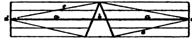
FIG. 42.—Wenham's system of Aeroplanes designed to carry a man. a, a , Thin planks, tapering at each end, and attached to a triangle. These are stretched five bands of holland 15 in. broad and 16 ft. long, the total length of the web being 80 ft. This apparatus when caught by a gust of wind, actually lifted the aeronaut. b , Similar plank for supporting the aeronaut. c, c , Thin bands of iron with truss planks a, a , and d, d , Vertical rods. Between
