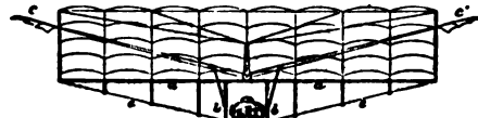
FIG. 43.—A similar system, planned by Wenham. a, a , Main spar 16 ft. long; b, b , Panels, with base board for aeronaut attached to main spar. These are stretched five webs of thin holland 15 in. broad. The aeroplanes are kept in parallel plane by vertical divisions of holland 2 ft. wide. c, c , Thin tie-band of steel with struts starting from main spar. This forms a strong light framework for the d, d , Wing propellers driven by the lect.
