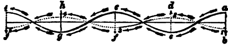
FIG. 29 shows how in progressive flight the wing and the body describe waded tracks,—the crests of the waves made by the wing (a, c, e, g, i) being placed opposite the crests of the waves made by the body 1, 2, 3, 4, 5).
